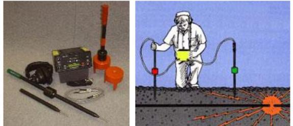
Ease and speed of fault finding with a thumper have been greatly enhanced with the addition of the S.D.A.D. to the Aqua-Tronics line. The Super DAD conveys more information about the fault location, and faster, with the addition of new microprocessor controlled electronics that provide bright, easier-to-see-and-read signals - day or night.
