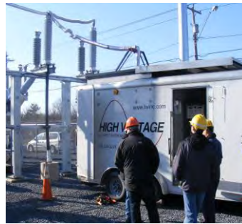
Van produced by HVI containing the VLF-200CMF with HV tank & controls in separate rooms and a 20 kW generator in separate section with noise deadening walls. Trailer top opens via motor driven chain system.
