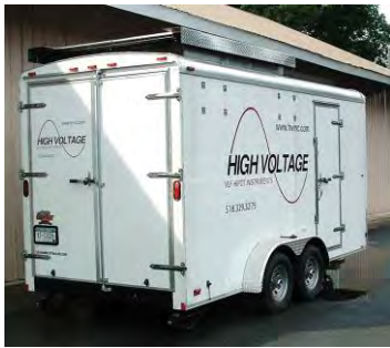
Van produced by HVI containing the VLF-200CMF with HV tank & controls in separate rooms and a 20 kW generator in separate section with noise deadening walls. Trailer top opens via motor driven chain system.
