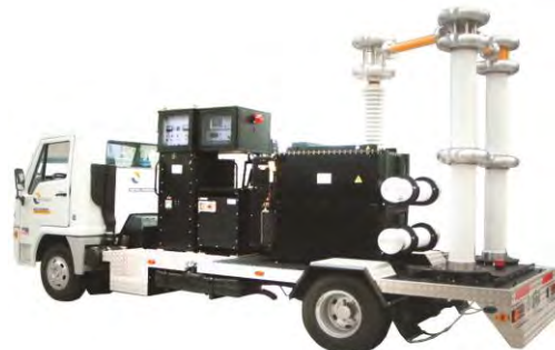
Truck produced by Inducor from Argentina with VLF-200CMF and generator. Partial Discharge and Tan Delta diagnostic cable testing products are provided by Power Diagnostix from Germany. Picture to the right is basic VLF-200CMF model.
