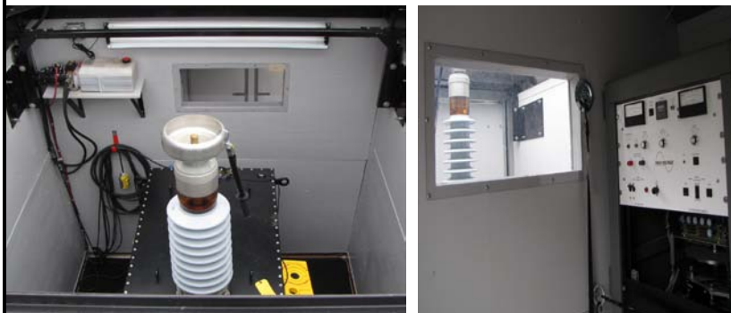
Trailer mounted VLF-200CMF. Includes retractable top to exit high voltage, separate room for controller, and 20 kW generator.
