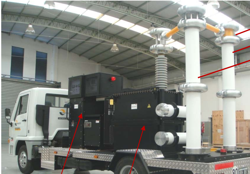
VLF Controls/regulator 200 kV VLF tank
