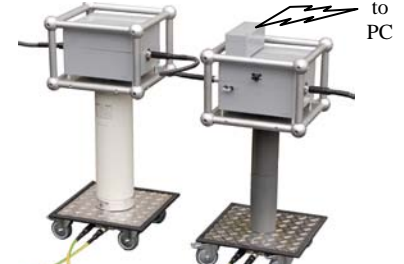
70 kV peak TD/PD system - PDIX 40 kV model also available
