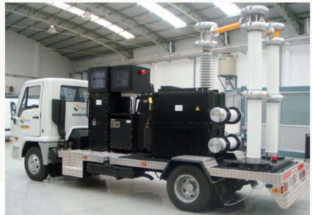
200kV VLF Withstand, VLF TD & VLF PD Test Truck Inducor Ingenieria S.A. Argentina
