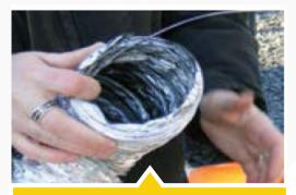
Small aluminum wire connecting load. Larger diameter aluminum dryer duct for limiting corona. Both must be isolated from ground for greater than the test voltage applied
