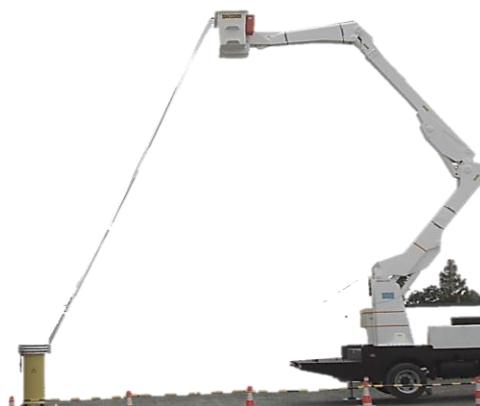
Model: ALT-300 in action 0 - 300 kVac @ 7 kVA
