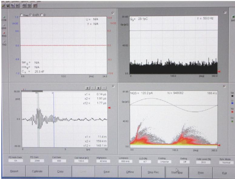
Many use PD detection as a comparative test. Many cables are tested and their level of PD activity compared. The worst offenders are dealt with first. If a comparative test is going to be used, it is much easier and less expensive to perform tan delta testing on the cables, or do both.
