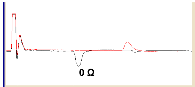
Short circuit Fault
