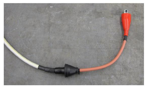
It is important to treat the entire unshielded (pink) part of the cable as if it was at high voltage. Never lay the pink insulation across a grounded surface or there is danger of insulation puncture. Also note that the white part of the cable is a plastic jacket layer over the grounded cable shield. Do not lay the pink part across the white part either.
