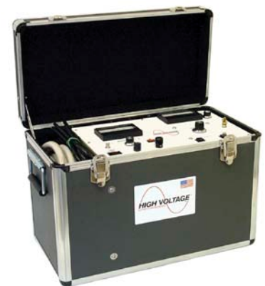
Model PFT-503CM 0 – 50 kVac @ 3 kVA 75lbs/34kg
