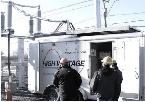
The below design includes a PD & TD cable diagnostic testing package (customer fabricated test truck)
