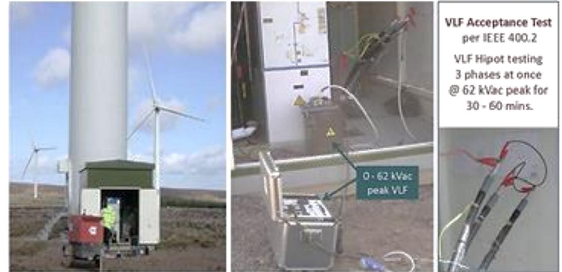
Cable system is new but needs **VLF Withstand** test to find faulty workmanship on splices and terminations and possible cable installation damage. Tan Delta and Partial Discharge testing are not needed. **VLF It!**
