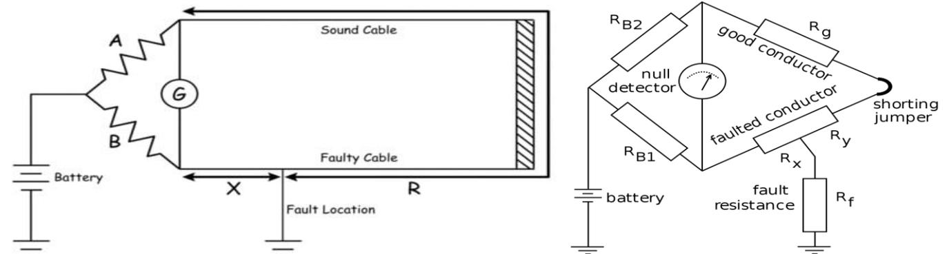
The *Shirla Sheath Test and Fault Location Device* from **Baur** uses the measuring bridge principle according to Murray and Glaser.
