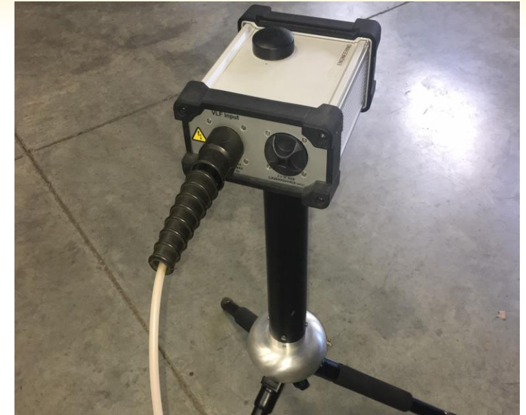
Push in MC Connector into socket and pigtail ground to ground stud
