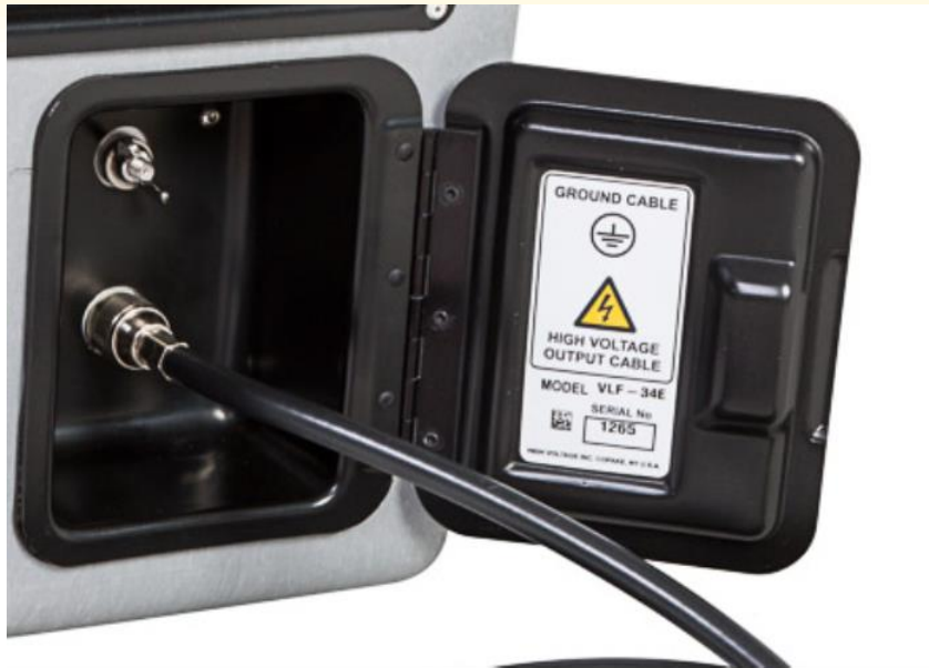
Install shielded output cable supplied with TD Bridge
