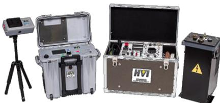
□ The **VLF & VLF E Series 0.1 Hz.** hipots are for testing loads of very high capacitance, like MV/HV power cables and large rotating machinery that would require hundreds of kVA of test power at 50/60 Hz. **Very Low Frequency (VLF) AC Technology** is available in model sizes from 30 kVac - 200 kVac, able to perform testing of loads from 0.1  $\mu$ F - 50  $\mu$ F. IEEE400.2-2013 & IEEE433-2012 apply. VLF TD and PD testing available.
