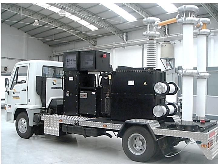
**200kV VLF Withstand, VLF TD & VLF PD Test Truck**
