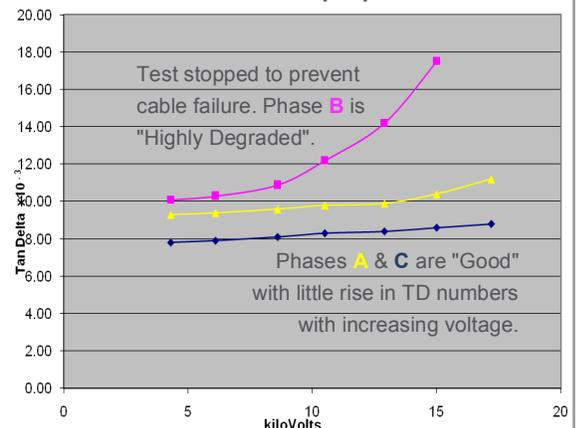
For example, if the curve trends sharply upward as the voltage is raised, the cable is highly degraded. Test many cables and rate them as **Highly Degraded, Moderately Degraded, or Good.** This, and other data and cable history, is used to help **prioritize cable replacement, injection, and/or what other tests** may be of value.
