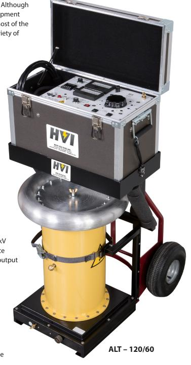
aerial lift industry and offers 0 to 120 kV for the boom test and a half-voltage, full-kVA tap that gives twice the output current up to 60 kV for the ac bucket liner test. We include a hand cart for portability and there is a 250 uA low current meter scale for precise leakage readings.
