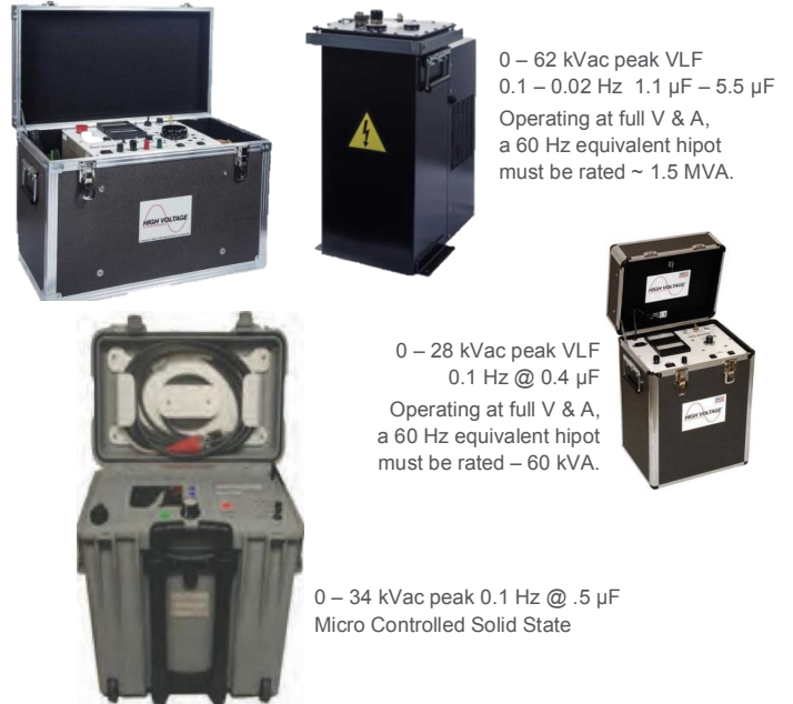
Fig. 6: Three VLF AC Hipot kVA Ratings vs. 60 Hz.
