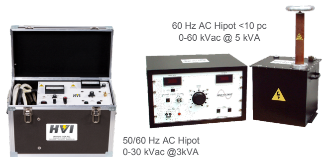
Fig. 3: Two AC Dielectric Test Sets
