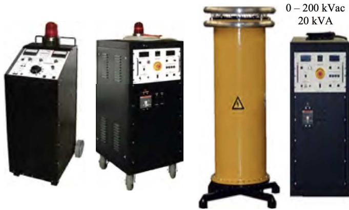
Fig. 4: Various AC Dielectric Test Sets
