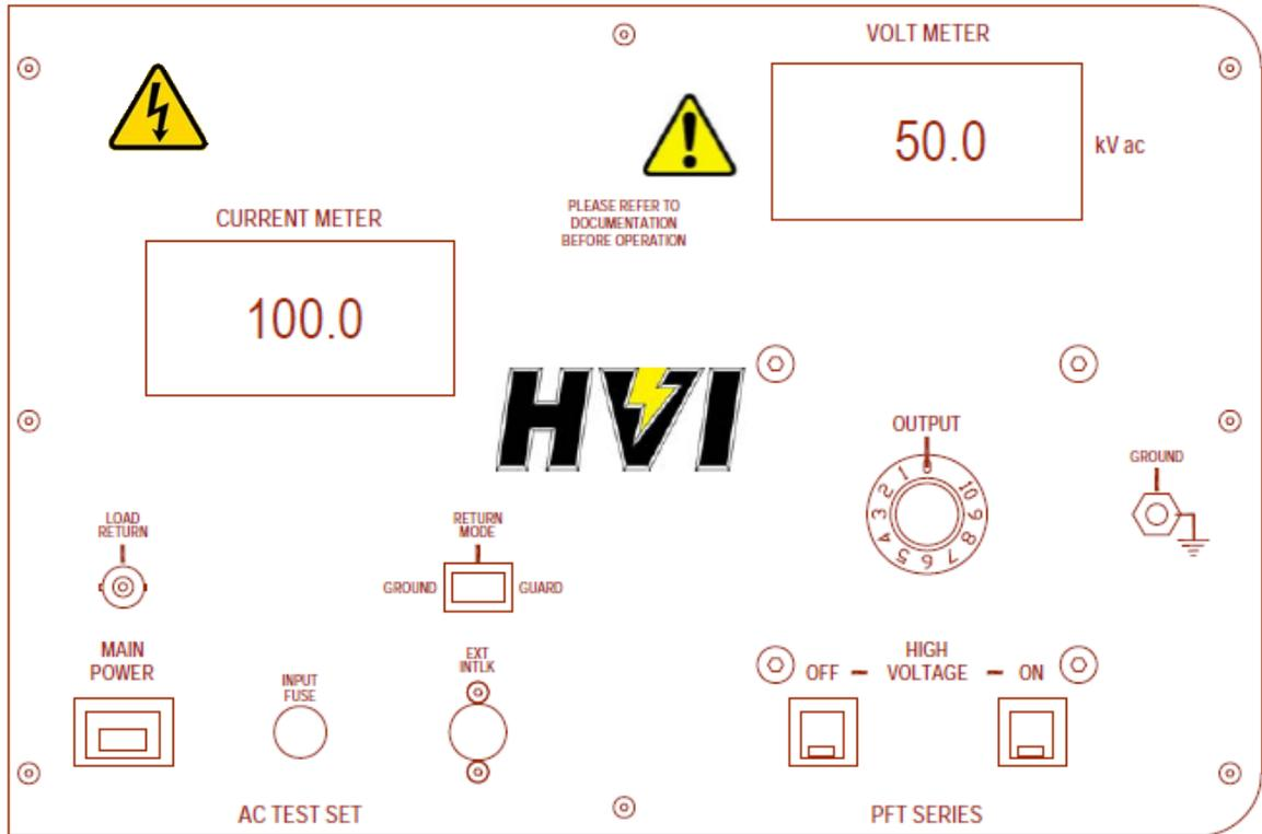
Figure 1A PFT DIGITAL Series front panel Controls
