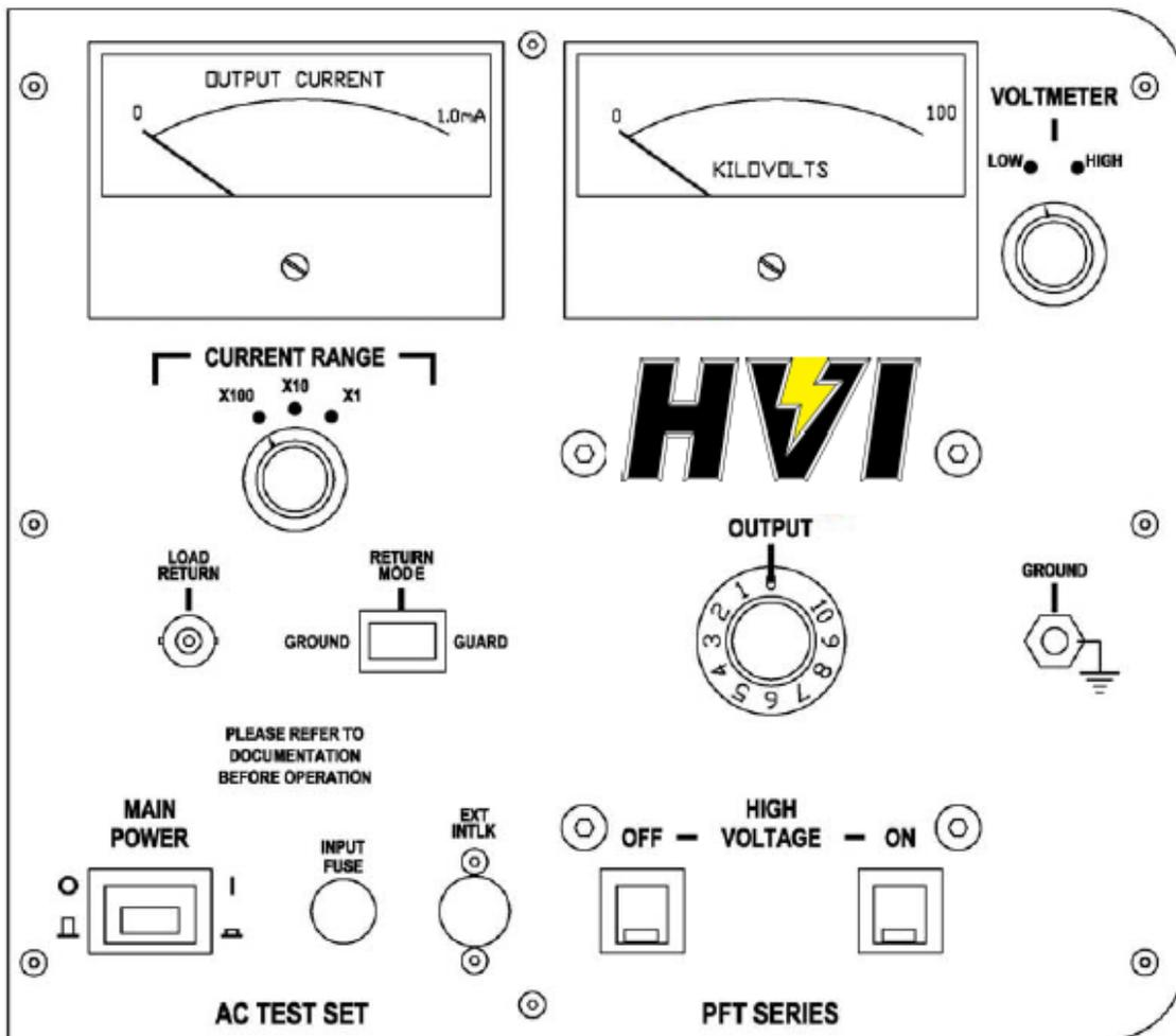
Figure 1C PFT-652/1003 Series front panel controls (Two Piece).
