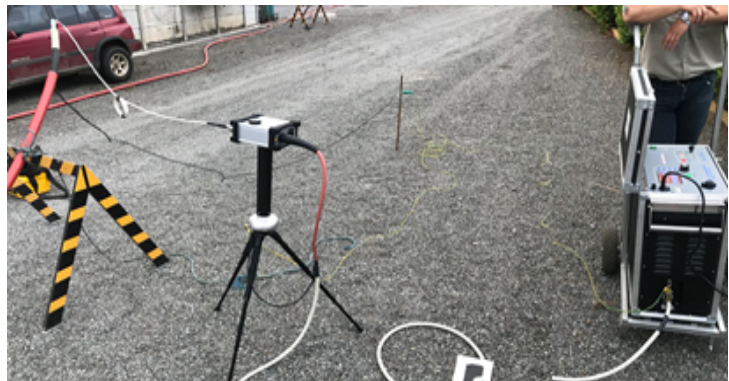
Testing a 35 kV cable
