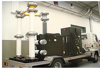
Van produced by HVI containing the VLF-200CMF with HV tank & controls in separate rooms and a 20 kW generator in separate section with noise deadening walls. Trailer top opens via motor driven chain system.
