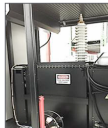
Custom container designed and produced by HVI to house VLF-200CMF. Top is motor driven to open.
