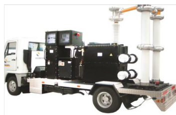
Van produced by HVI containing the VLF-200CMF with HV tank & controls in separate rooms and a 20 kW generator in separate section with noise deadening walls. Trailer top opens via motor driven chain system.
