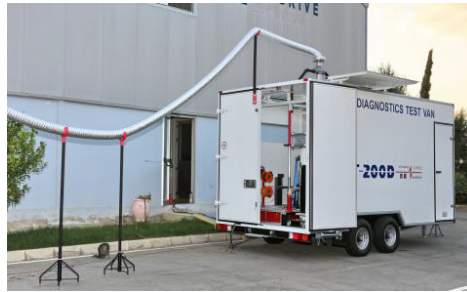
Diagnostix PD and TD measurement equipment. Top opens to expose HV output.
