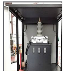
Custom container designed and produced by HVI to house VLF-200CMF. Top is motor driven to open.
