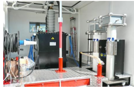
Diagnostix PD and TD measurement equipment. Top opens to expose HV output.
