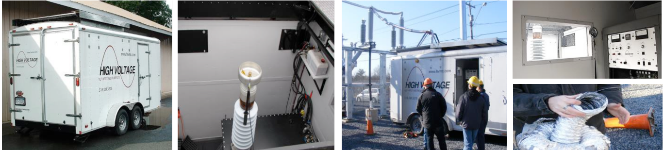
Van produced by HVI containing the VLF-200CMF with HV tank & controls in separate rooms and a 20 kW generator in separate section with noise deadening walls. Trailer top opens via motor driven chain system.
