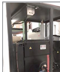
Custom container designed and produced by HVI to house VLF-200CMF. Top is motor driven to open.
