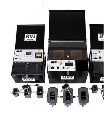
voltage of insulating oils used in electrical equipment. These lightweight, rugged units are designed for field and laboratory use. They feature fully preprogrammed sequences for commonly used ASTM oil tests, including ASTM D1816/2012, ASTM D877/2013 and IEC 156/1995. They also allow for custom programming, and results can be save directly to the device and/or exported to a computer.
