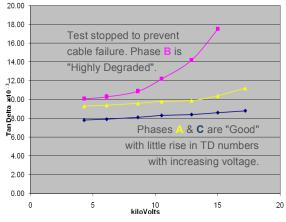
easily measured and assumptions can be made about the degree of degradation. For example, if the curve trends sharply upward as the voltage is raised, the cable is highly degraded. Test many cables and rate them as **Highly Degraded**, **Moderately Degraded**, or **Good**. This, and other data and cable history, is used to help **prioritize cable replacement**, **injection**, and/or what **other tests** may be of value.
