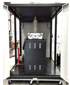
Custom container designed and produced by HVI to house VLF-200CMF. Top is motor driven to open for HV output.
