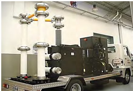
Truck produced by Inducor from Argentina with VLF-200CMF and generator. Partial Discharge and Tan Delta diagnostic cable testing products are provided by Power Diagnostix from Germany. Picture to the right is basic VLF-200CMF model.
