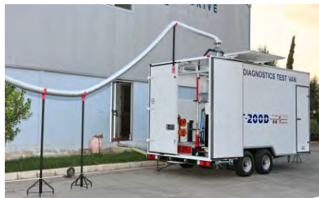
Trailer produced by Vital Drive from Cypress. Includes VLF-200CMF and Power Diagnostix PD and TD measurement equipment. Top opens to expose HV output.
