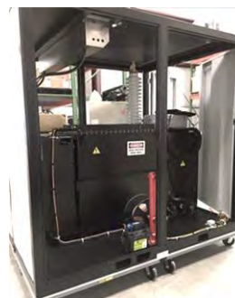
Custom container designed and produced by HVI to house VLF-200CMF. Top is motor driven to open for HV output.
