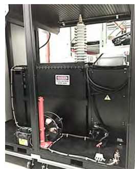
Custom container designed and produced by HVI to house VLF-200CMF. Top is motor driven to open for HV output.
