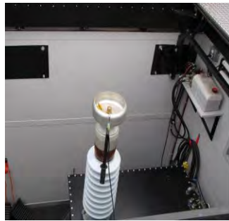
Van produced by HVI containing the VLF-200CMF with HV tank & controls in separate rooms and a 20 kW generator in separate section with noise deadening walls. Trailer top opens via motor driven chain system.
