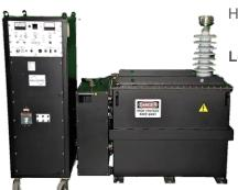
Controller/Regulator: 23" w x 30" d x 62" h (61 x 76 x 157 cm) 750 lbs. (340kg) HV Tank Section: 61" w x 37" d x 61" h (150 x 94 x 221 cm) 2555 lbs. (1160kg) HV Output: Oil Filled Porcelain Bushing @ 250kV BIL Rating
